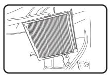
2: Lift front of cover to remove, turn cover over to remove filter.
