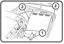
1: Open engine hood to vertical position. Unscrew plastic nut (1). Release both snap fastners (2) on filter housing.
